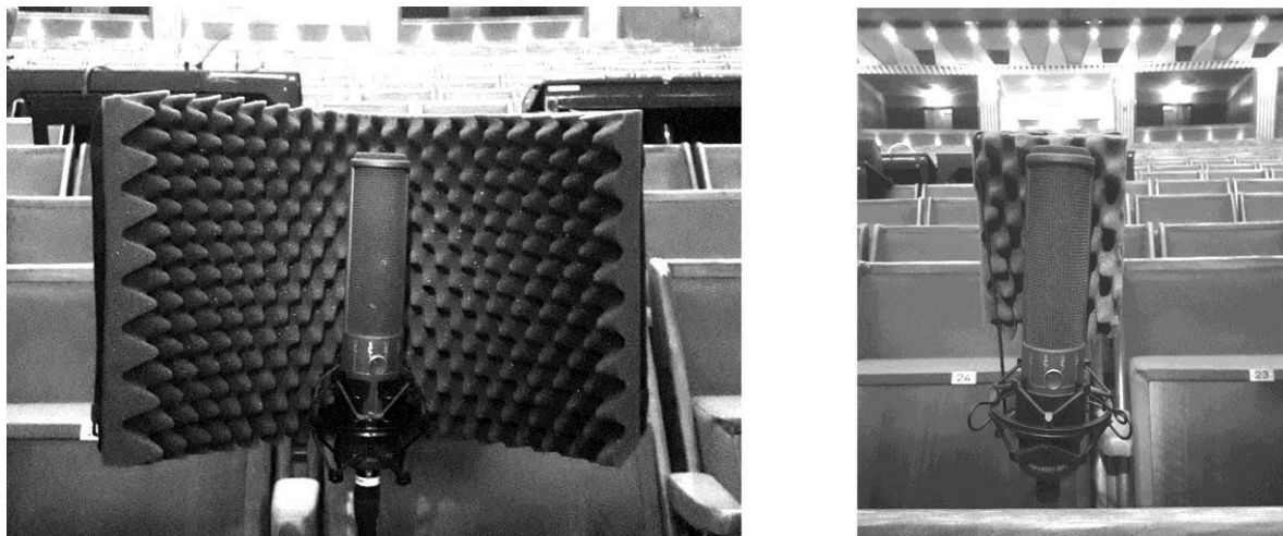
Fig. 14: (left) “ACOUSTILITE” - absorptive panel (normal size) and (right) “ACOUSTILITE MINI” panel
